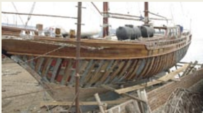
A gulet being replanked in a Bodrum boatyard
